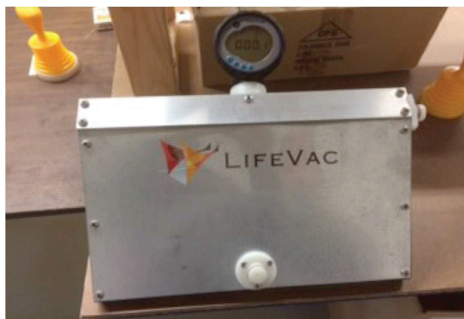
Figure 1. Vacuum testing fixture used in LifeVac testing.
